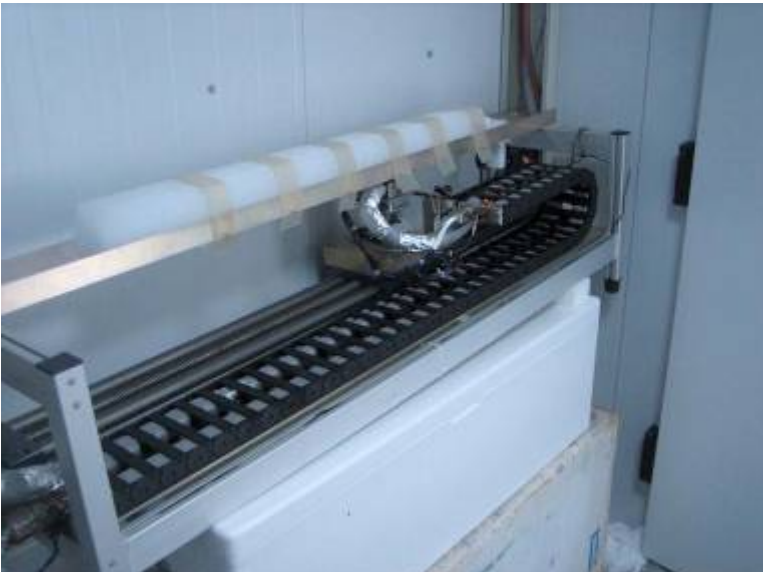
Fig. 2.7 - The finger melter in action at Dome C. This prototype is designed to resample ice cores in the field for allowing a continuous chemical analysis of the core.
