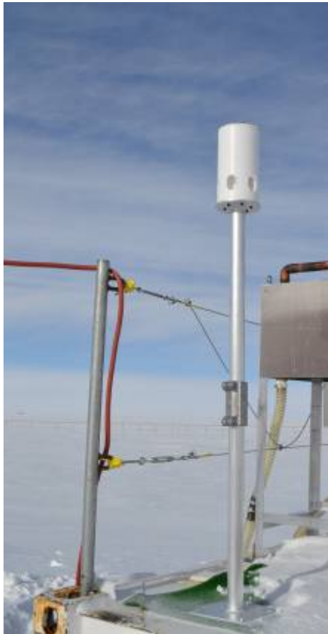
Photo 1 - Sampling system (all Teflon made) installed on the roof top of the container glacio at DC
