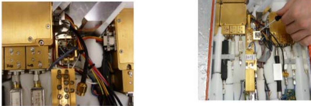
Fig. 2.5 - Noise diode prior to its replacement (left) and during (right).
