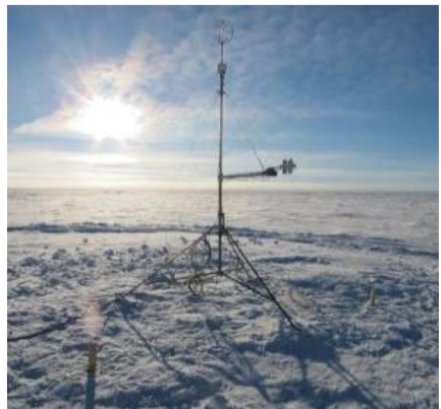
Fig. A3.2 - Micrometeo Mast with sonic anemometer and net radiometer at Dome C.
