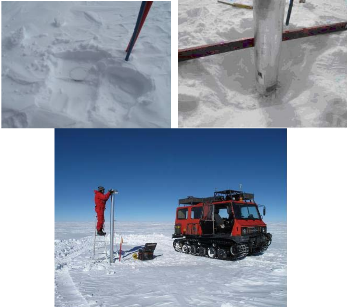
Fig. A2.4 – Discovering of old pole’s top buried in the snow, installation of the extension, and stationing of the GPS antenna on the top of the new pole.
