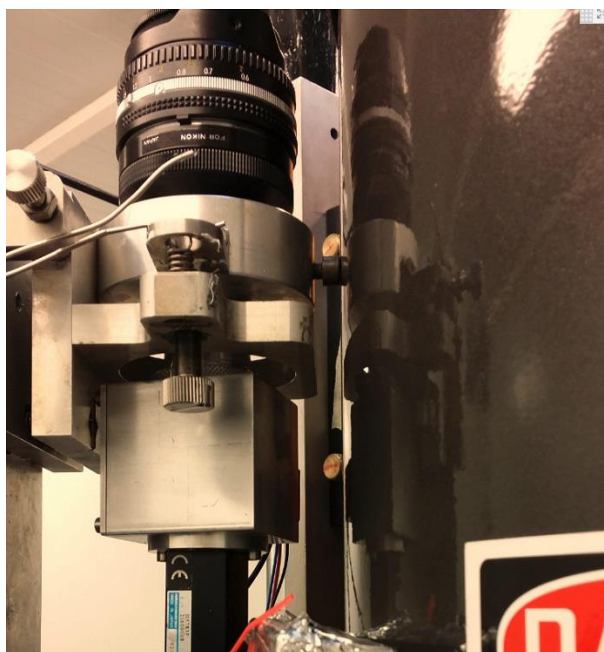
Figure X – Two channels 50mm f/2 tropospheric lidar receiver allowing for backscattering measurements in the range 5-25km
