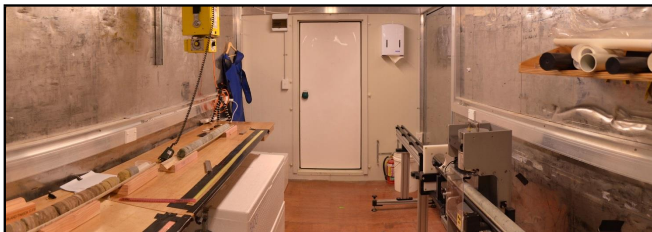
Figure 2 - Interior of the cold laboratory, showing cores on logging and X-ray tables, portable X-ray unit, protective lead apron for X-ray operator, core storage boxes, and Geotek multi-sensor core logger, including core track, magnetic susceptibility measurement loop, and gamma-ray source and detector. The plastic cylinders on the far right are thickness standards for calibrating the core logger.
