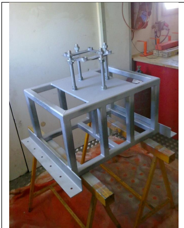
Metal pedestal for AWS520 (made by Pierre Pejoine)
