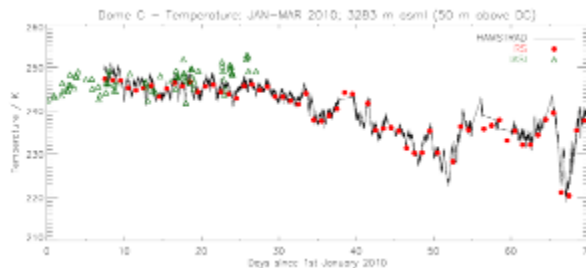
Time evolution of temperature from 1 st January to mid-March 2010 as measured by HAMSTRAD (black line) and by the radiosondes (red circles) at 50 m altitude above Dome C together with IASI space-borne measurements (green triangles) in January 2010.
