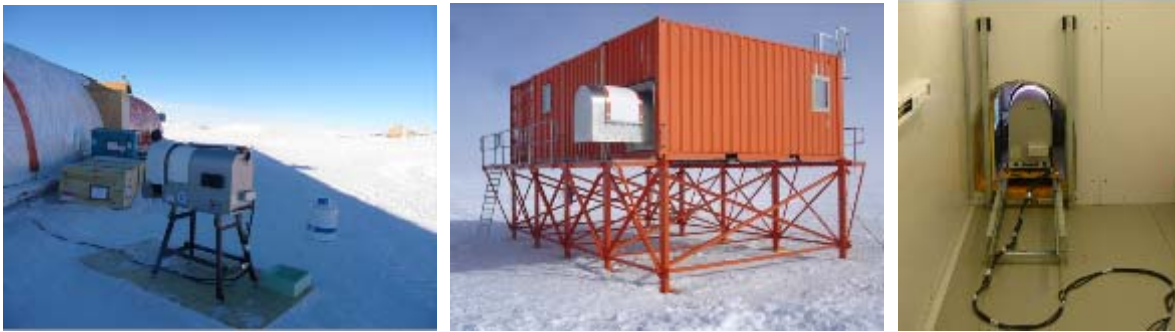
The HAMSTRAD instrument deployed outside at Dome C (left). The shelter with the external shield containing the HAMSTRAD radiometer (center). The HAMSTRAD instrument inside the shelter on the rails within the shield (right).
