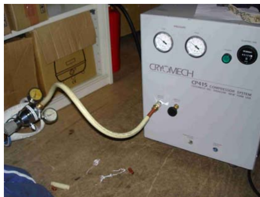
He bottle connected to the He compressor via the pres-sure reducer when attempting to refill the He
