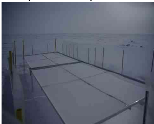
Photo 2.1 - Example of one of the field under study. The plexiglas plates allow or not the UV light to penetrate the underlying snow
