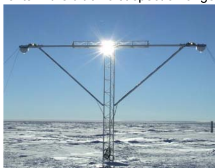
The albedo rack for measurements of upwelling-fluxes and albedo.
