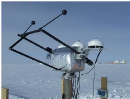
The tracker system hosting downwelling measurements
