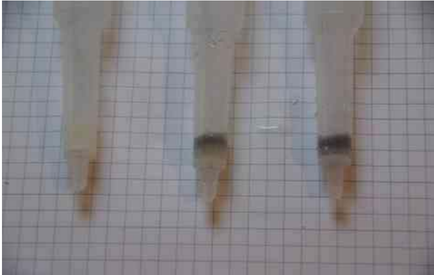
Photo 2.3 - Difference in colour of our filtration units between a deep sample (clean) and surface samples collected in the clean area. Obviously, the “clean area” is not so clean!
