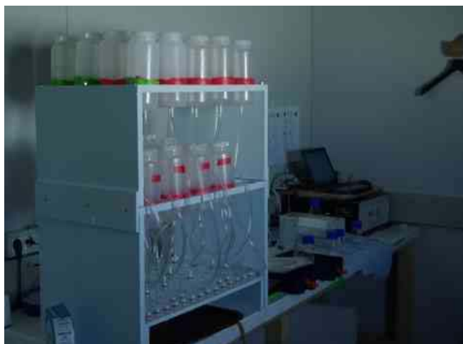
Photo 2.2 - Laboratory set up in the warm EPICA laboratory, showing the extraction apparatus (to isolate the nitrate before analysis in Grenoble) and the CFA in the back (for concentration measurements).
