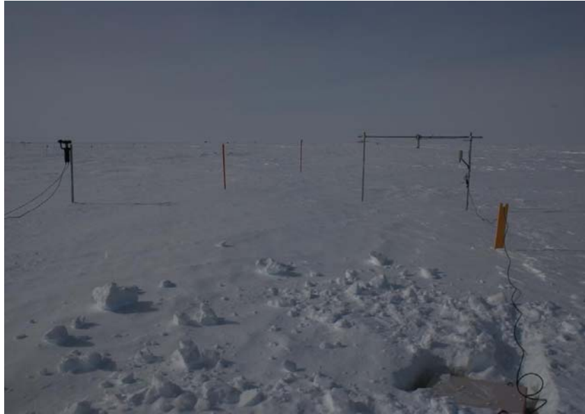
Fig. 2.17 - Weather sensor, sonic ranger depth and accumulation stakes. 18 January 2008. Photo D. Six
