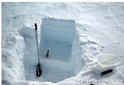
50 cm snow pit dug with a sample collected every 2 cm
