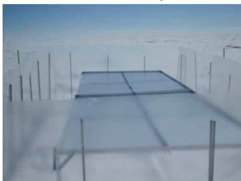
Example of a snow field delimited by stack and with its plexiglas cover
