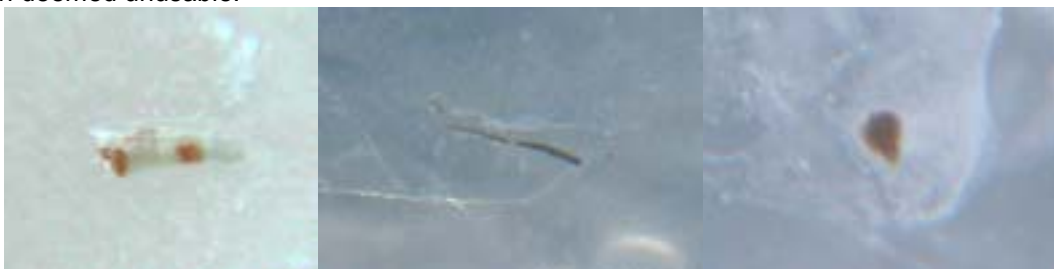
3 types of inclusions. Sizes are about 2 mm, 10 mm, 1 mm from left to right.
