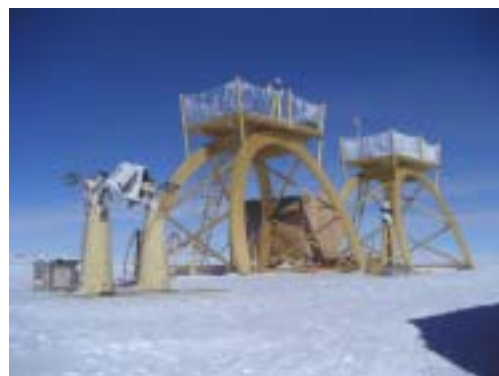
View of the ConcordiAstro observatory in December 2004. The DIMM is on top of the plat-form, GSM is the twin telescopes on the ground. The wooden igloo is between the two platforms
