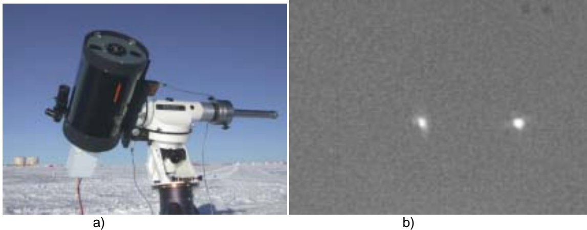
Fig. 2.7 - a) the DIMM system operating at the astrophysics tent in the first days of the mission. Note the two hole mask at the telescope top. The white box at telescope back contains the camera. b) typical short-exposure frame at the focus. The 2 images move with turbulence, analysis of their differential motion give the turbulence parameters.
