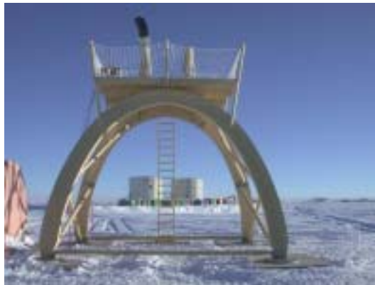
Fig. 2.5 - Site-testing platform. The telescope operating at the top of the platform. A laboratory (computer, acquisition system) had been set up in the adjacent tent (on the left).
